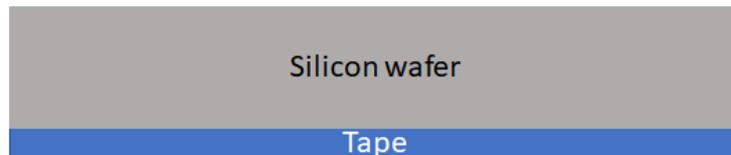
3. Wafer thinning (Grinding) from the backside
